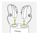
(j) Do not hold the tubes when removing the hearing aids from the charger as this can damage the tube.
